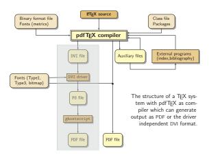
Figure 1: The traditional way of creating PDF output, via DVI.
