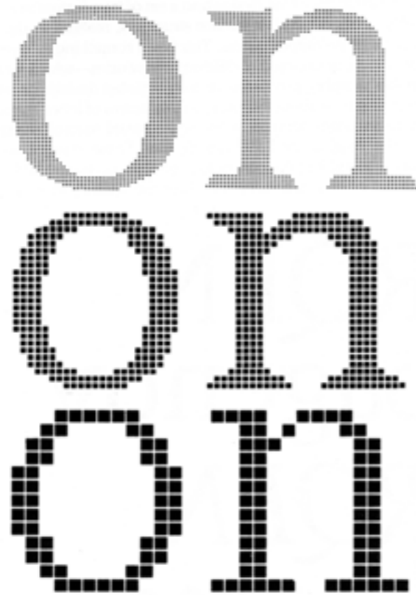
Sample digitizations of 'o' and 'n.' As the resolution decreases, the design changes but maintains certain formal characteristics. Top to bottom: 100 x 100 pixels per em; 50 x 50 pixels per em; 25 x 25 pixels per em.
